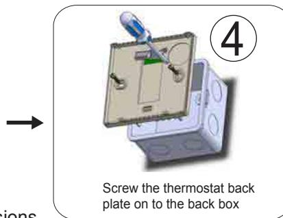
Screw the thermostat back plate on to the back box
