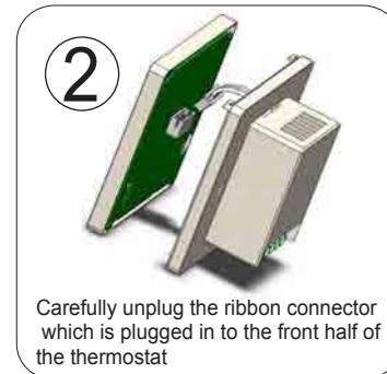
Carefully unplug the ribbon connector which is plugged in to the front half of the thermostat
