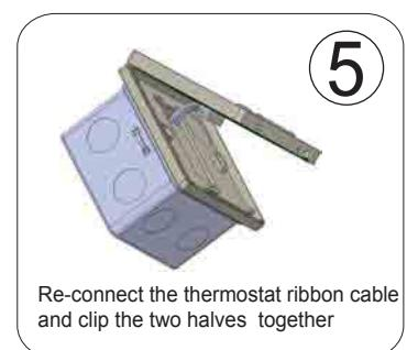
Re-connect the thermostat ribbon cable and clip the two halves together
