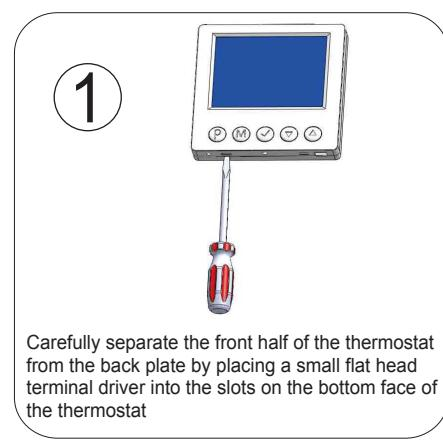
Carefully separate the front half of the thermostat from the back plate by placing a small flat head terminal driver into the slots on the bottom face of the thermostat
