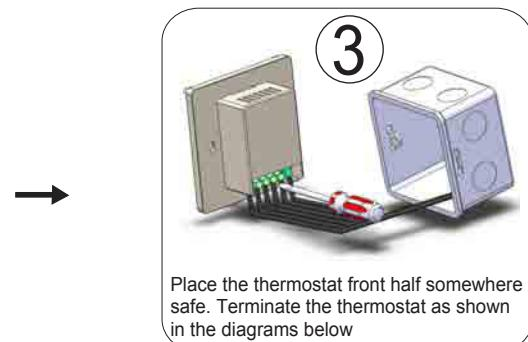
Place the thermostat front half somewhere safe. Terminate the thermostat as shown in the diagrams below
