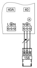
Fig. 15 Example: Power supply with plug 156
