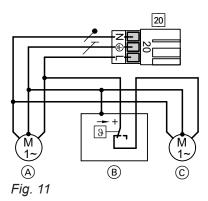
The common power consumption of both pumps must **not exceed 1 A**.
