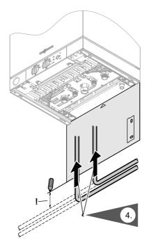
4. Only if a DHW cylinder is installed adjacent to the boiler: Route the connection lines to the DHW cylinder below the sub-mounting kit. Using the drilling template supplied, prepare the layout of the connection lines.
