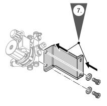
**7.** Secure the mounting bracket to the mixer casing with the screws and washers supplied.
