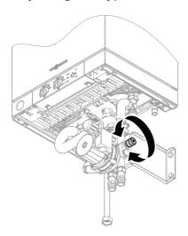
A bypass is integrated into the heating circuit with mixer. In the delivered condition, the bypass is closed. If required, open the bypass to minimise temperature peaks (by turning it anti-clockwise).
