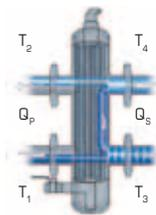
In this situation, demand is greater than supply. This will cause the ΔT between T<sub>3</sub> and T<sub>4</sub> to drop. Some of the return water will join the supply, as a result of which it will take longer for the rooms to reach their set temperature. Where possible, the power of the boiler or cooler will then be increased.
