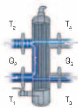
In the third situation, supply is greater than demand. This will cause the ΔT between T<sub>1</sub> and T<sub>2</sub> to drop. Some of the supply water will now join the return water, as a result of which the efficiency of the boiler or cooler will decrease. Where possible, the power will be modulated downwards.
