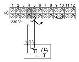
(A) Terminal strip inside the Vitotronic 100, type KC3
