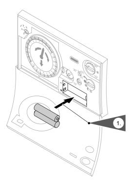
**1.** Insert batteries into the battery compartment (observe correct polarity).
