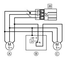
The common power consumption of both pumps must **not exceed 2 A**.
