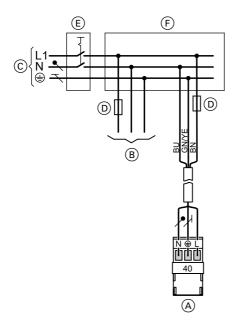
Make the mains connection in accordance with the diagram.
