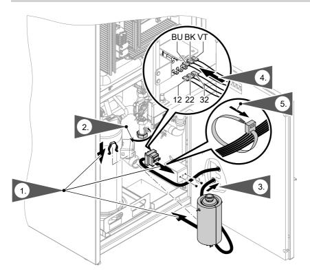
**Notes on steps 1 and 2:** Ensure the O-ring and flat gasket are seated correctly.
