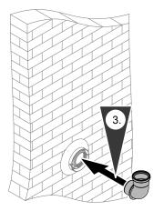
**3.** Push the flue bend into the external wall connection.
