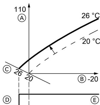
Fig. 26 Adjusting the standard set room temperature from  $20\text{ }^{\circ}\text{C}$  to  $26\text{ }^{\circ}\text{C}$
