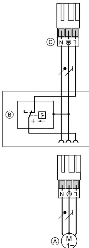
Electromechanical temperature limiter using the liquid expansion principle
