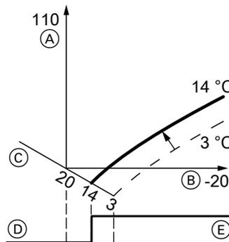
Fig. 27 Adjusting the reduced set room temperature from  $3\text{ }^{\circ}\text{C}$  to  $14\text{ }^{\circ}\text{C}$
