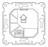
Insert the thermostat into the surface box with the arrow pointing upwards and secure with the screws provided.
