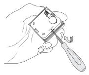
**3.** Use a screwdriver to carefully remove the front cover from the back panel.
