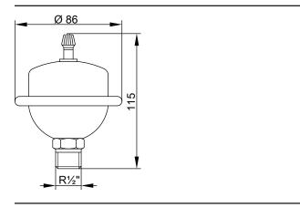
If the pipework to which the Vitodens is connected also supplies draw-off points at which water hammers may occur (e.g. pressure washers, washing machines or dishwashers): Install shock arrestors near the source of the water hammer (recommended).
