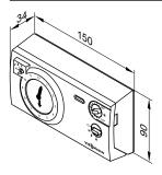
IP 20 to EN 60529 Ensure through design/installation
