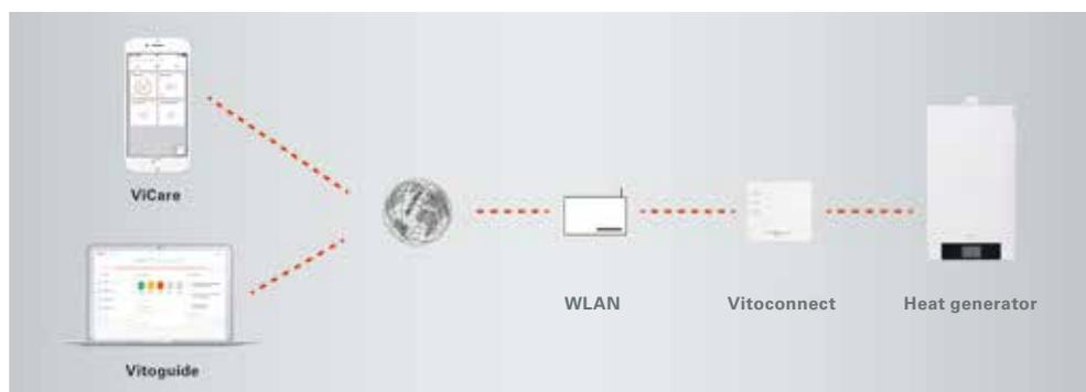
ViCare accesses the Vitoconnect online interface to control the heat generator. Once the system user has given their consent, the contractor can use Vitoguide to keep a constant eye on their customer's system.
