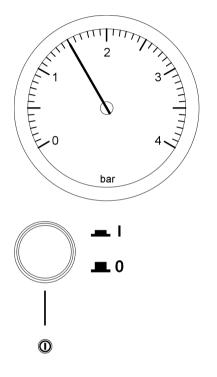
Check the pressure of your heating system on the pressure gauge.
