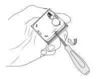
Use a screwdriver to carefully remove the front cover from the back panel.
