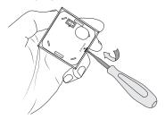
Press the screwdriver into the groove on the underside and lift the front section upwards until you hear a "click". 2. Lift off the front section and frame.
