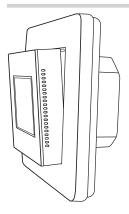
Place on the frame. First hook the front section in at the bottom and then press it in at the top until it audibly engages.
