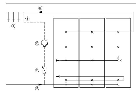
Connection in conjunction with a district heating system without return temperature limit or in conjunction with boilers (low temperature operation) and a simple DHW circulation pipe
