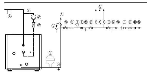
Connection on the DHW side to DIN 1988
