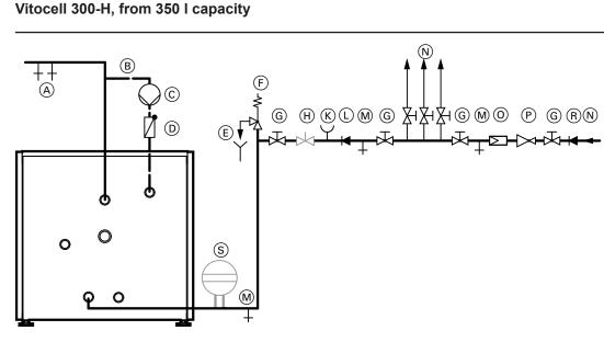
Connection on the DHW side to DIN 1988
