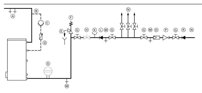
Connection on the DHW side in accordance with DIN 1988
