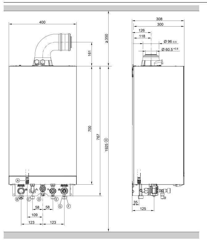
Illustration shows a gas condensing combi boiler
