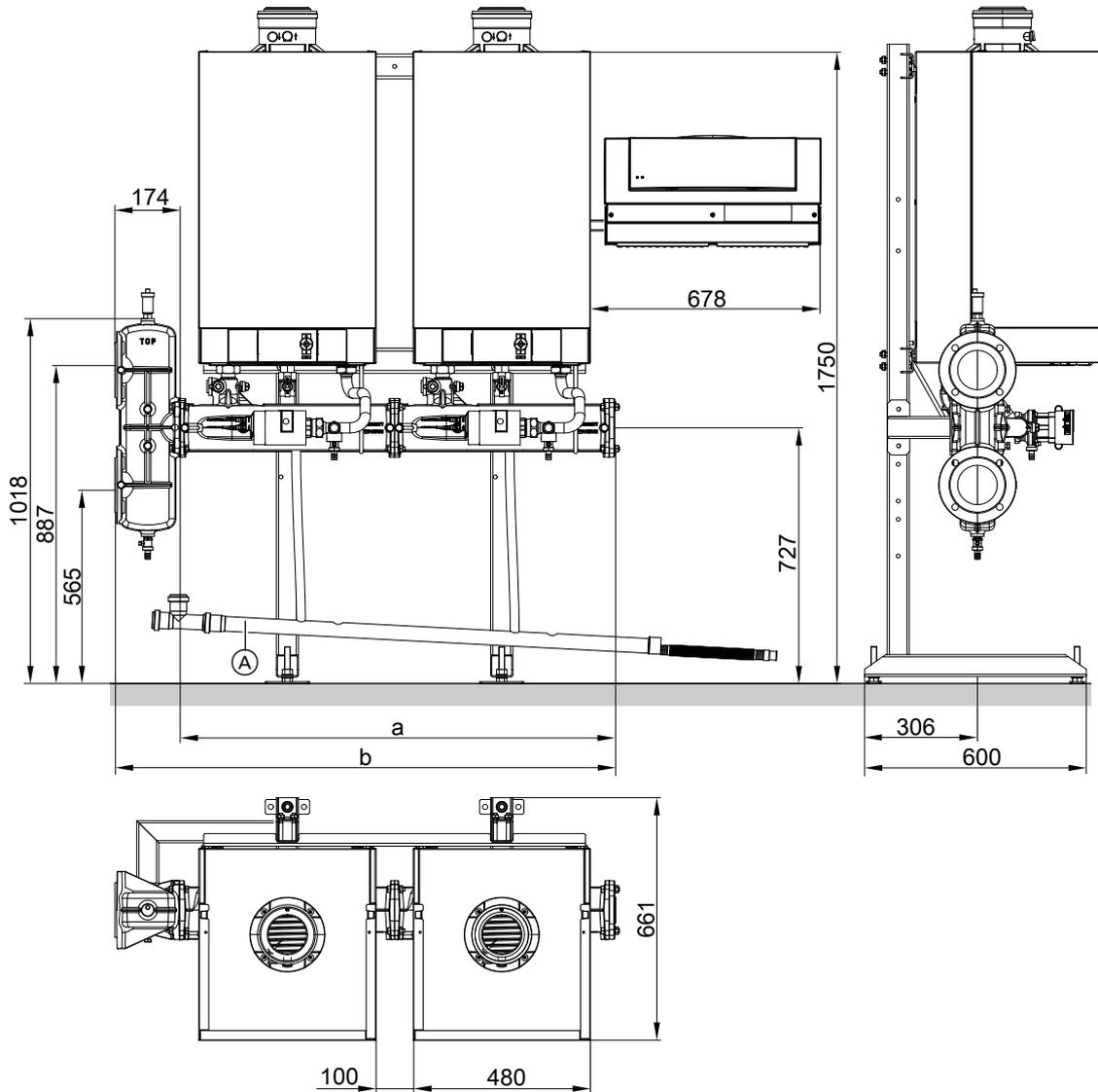
Shown without the thermal insulation supplied
