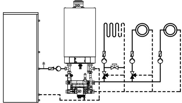
If the cylinder capacity is below the following values, we recommend connecting the DHW cylinder downstream of the low loss header in the secondary side of the heating system.
