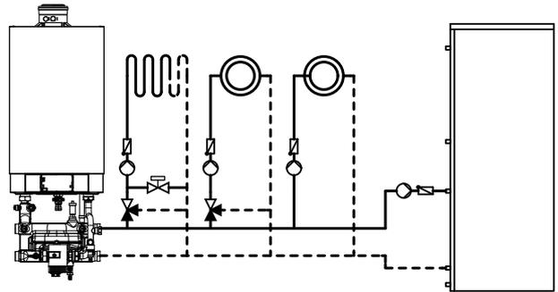
In conjunction with multi boiler systems, the DHW cylinder must be connected downstream of the low loss header on the secondary side of the heating system.
