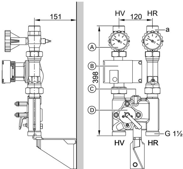
Divicon with mixer (wall mounting, shown without thermal insulation or mixer drive extension kit)
