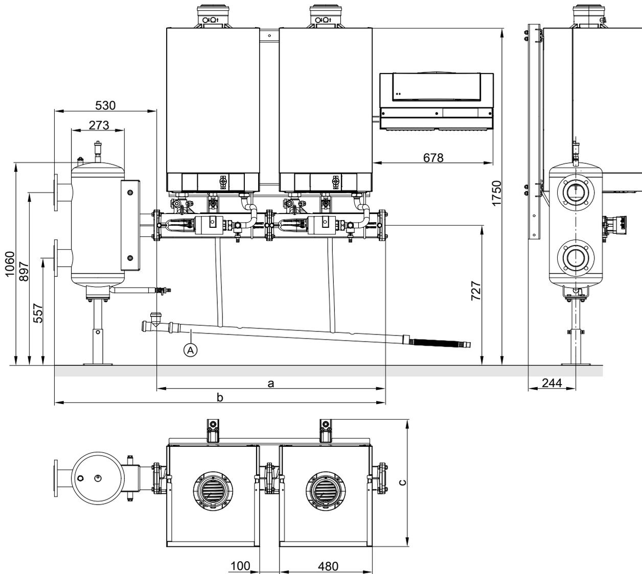
Shown without the thermal insulation supplied
