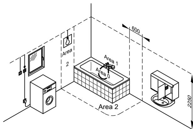
Electrical equipment in rooms containing a bathtub or a shower must be installed in such a way that users cannot be exposed to dangerous body currents. VDE 0100 specifies that cables supplying permanently installed consumers in zones 1 and 2 should only be run vertically and routed into the equipment from the back.
