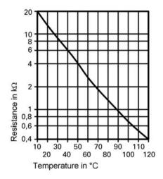
**3.** Replace the sensor in case of severe deviation.
