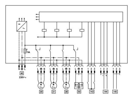
The external extension is connected to the boiler control unit via the KM BUS. The following functions can be controlled or processed simultaneously via the extension:
