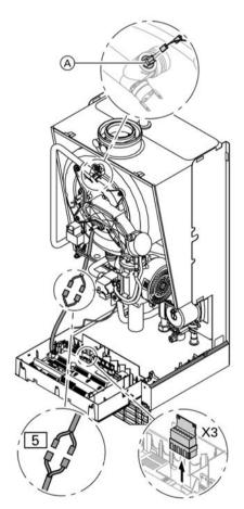
1. Boiler temperature sensor: Pull the leads from boiler temperature sensor (A) and measure the resistance.
