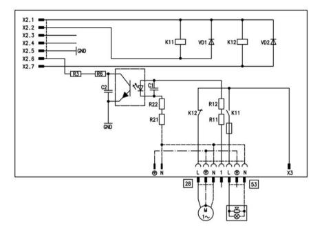
The internal extension is integrated into the control unit housing. As alternative, the following functions can be connected to relay output [28]. The function is allocated via coding address 53:
