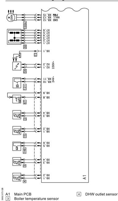
Connection and wiring diagrams – internal connections
