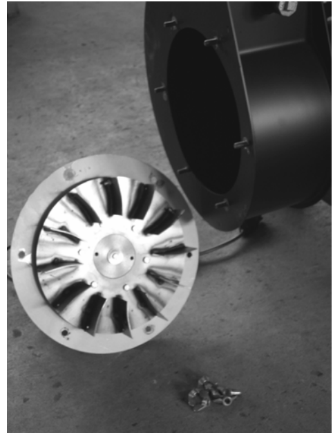
Fig. 15 Motor with impellor, detached
