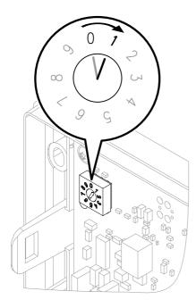
If several mixer extension kits are being connected, set rotary switch S1.
