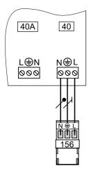
Create the power supply connection. Route the power cable to the heat generator control unit and connect to plug 156].
