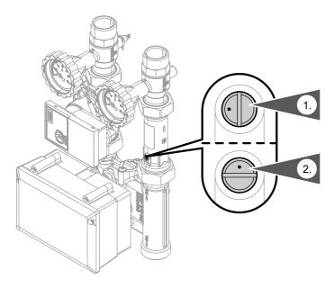
1. For filling (with heating water), open the check valve in the heating return by positioning the slot of the screw in the vertical position.
