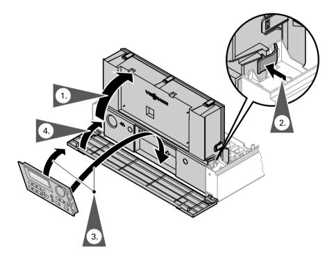
Closing control unit housing and inserting user interface
