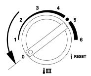
Turn rotary selector "Ⅲ ♣" anticlockwise within 2 s.
