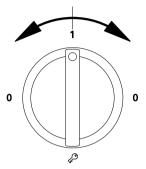
Adjust the control unit to natural gas or LPG by turning the rotary selector
