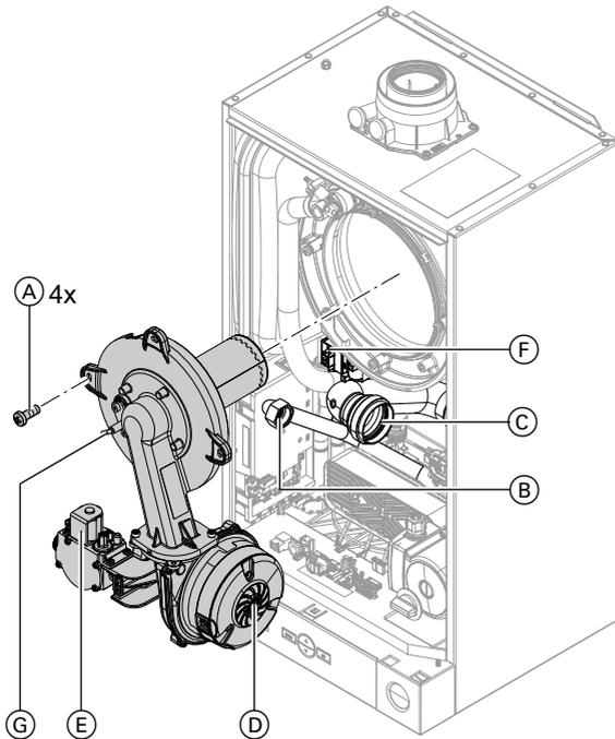
1. Fit burner and tighten 4 screws (A) diagonally.
