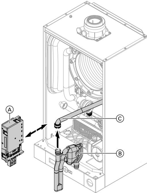
1. Unclip burner control unit (A) and remove. Protect against escaping condensate.
