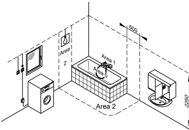
The Vitodens is approved for installation in wet rooms (e.g. bathroom or shower rooms) (protection IP X4 D, splash-proof).
