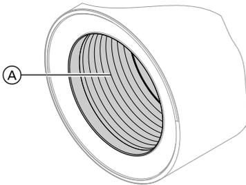
1. Use a vacuum cleaner to remove combustion residues from heating surface (A) of the heat exchanger.
