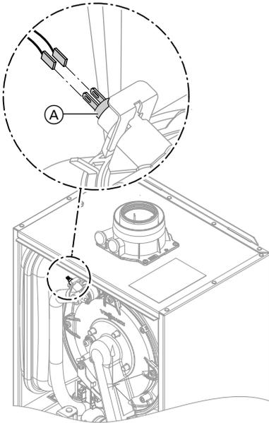
1. Pull out the leads on boiler water temperature sensor (A) and check the resistance.
