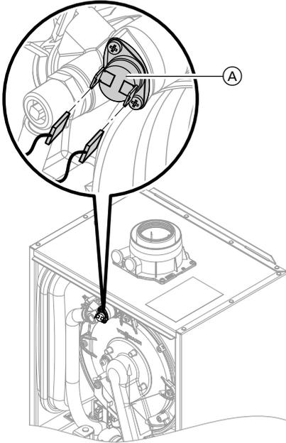
If the burner control unit cannot be reset after a fault shutdown although the boiler water temperature is below approx. 95 °C, check the temperature limiter.
