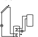
When exceeding the set cylinder temperature "S SL" (see page 52) the transfer pump R2 will start.
