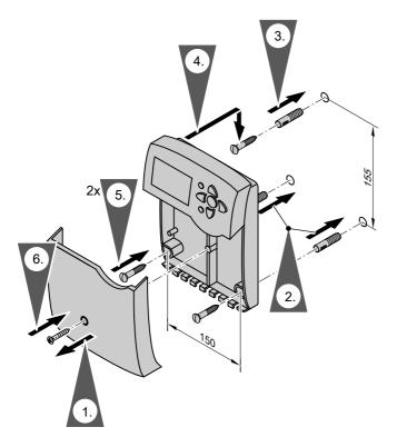
Before closing the solar control unit, make all electrical connections and apply a strain relief to all cables/leads.
