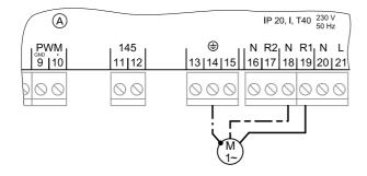
(A) Wiring chamber of the solar control R1 Solar circuit pump unit
