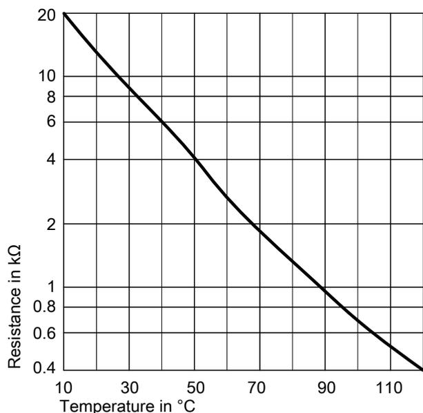
Fig. 51 Sensor type: NTC 10 kΩ
