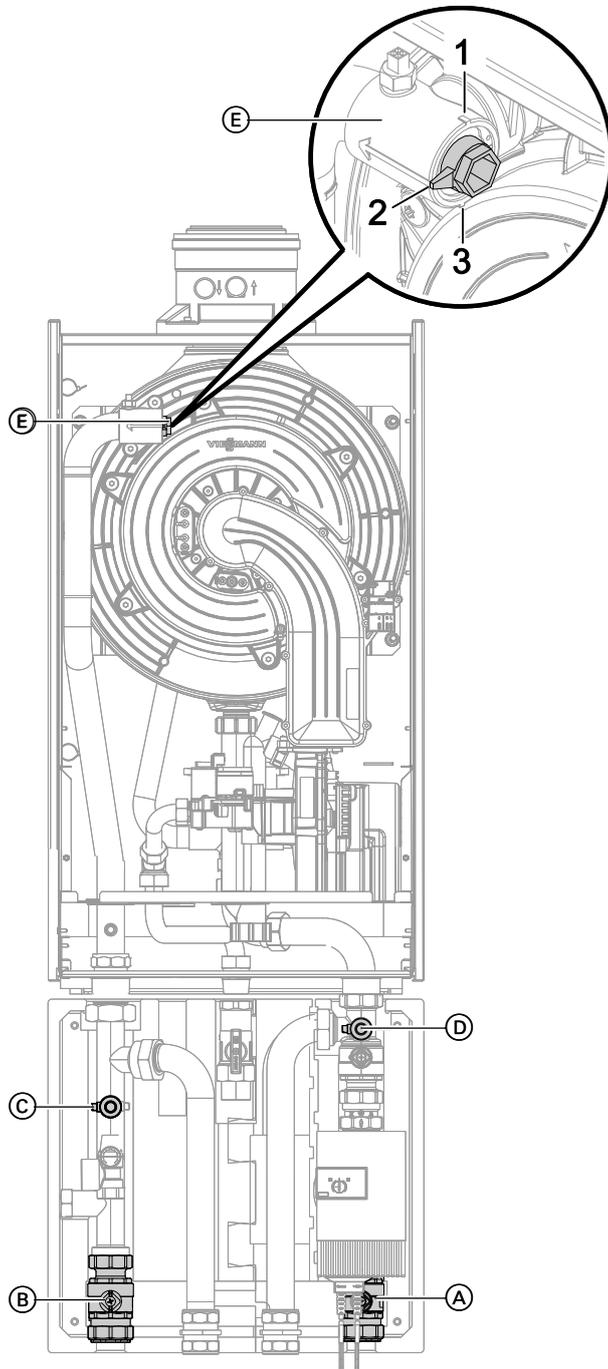
1. Close shut-off valves (A) and (B).
