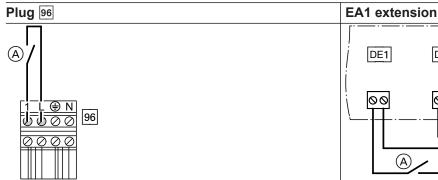
A Floating contact (when connecting, remove jumper between L and 1)
