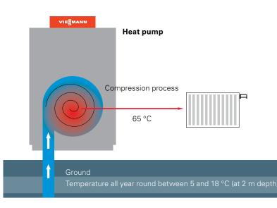
Getting hotter towards the centre: at an initial temperature of between 5 and 18 °C, a flow temperature of up to 72 °C is reached.
