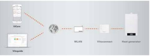
ViCare accesses the Vitoconnect online interface to control the heat generator. Once the system user has given their consent, the contractor can use Vitoguide to keep a constant eye on their customer's system.
