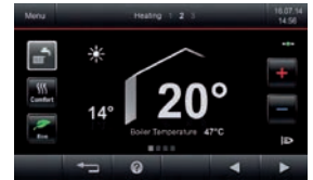
5 inch colour touchscreen control with energy cockpit (see page 26)
