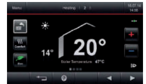
Weather compensation control features a 5" colour touchscreen with energy cockpit
