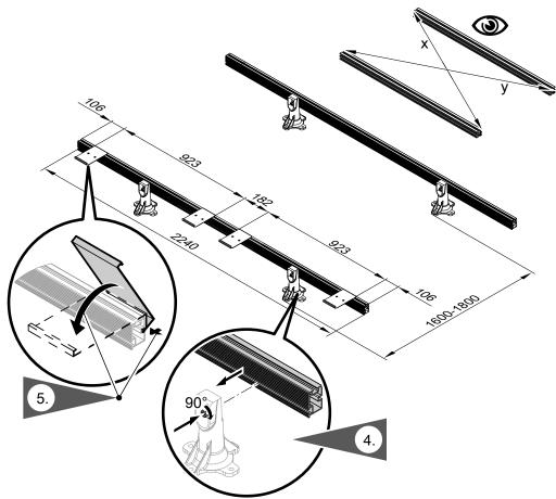
Fig. 9 Maximum deviation from dimensions x and y 10 mm
