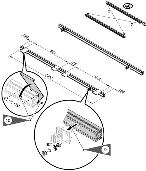
Fig. 31 Maximum deviation from dimensions x and y 10 mm
