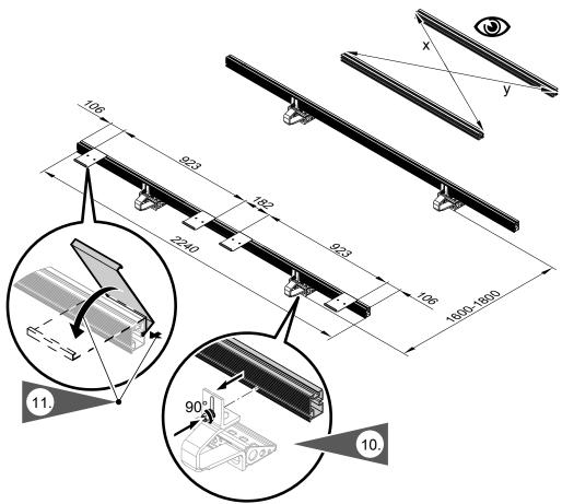
Fig. 5 Maximum deviation from dimensions x and y 10 mm
