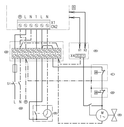
With Viessmann Vitotrol 100, RF/RF2 or standard room thermostat
