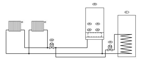
Radiators ® Boiler © DHW-cylinder @ Motorised valve ® Pump® Gauge@ Expansion vessel@ Savety valve
