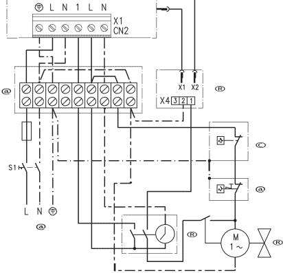
Terminals in the control unit © Cylinder demand terminal box © Cylinder thermostat @ Safety temperature sensor ® Valve
