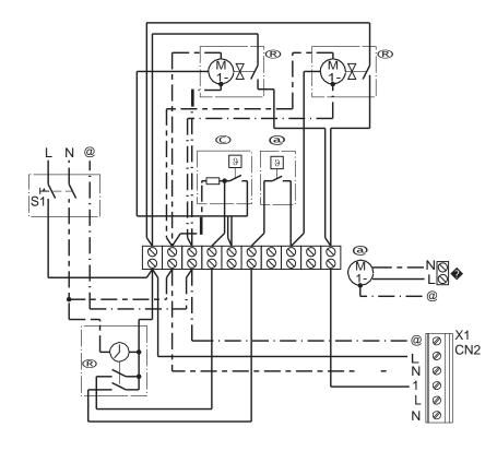
Power supply 230 V, 50 Hz ® Time controller © Roomthermostat (clock thermostat) @ Cylinder thermostat ® Zone valve
