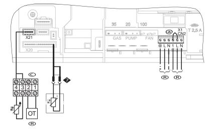
Tank sensor connection (sensor is optional - part no. 7178 348)
