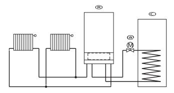
© DHW-cylinder @ Motorised valve (Energy cut-out)
