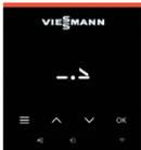
After completing the last setting, the 'End' symbol appears in the display. Confirm with 'OK' to start the flue gas temperature sensor test and 'Fst' is shown in the display. The system carries out a restart.
