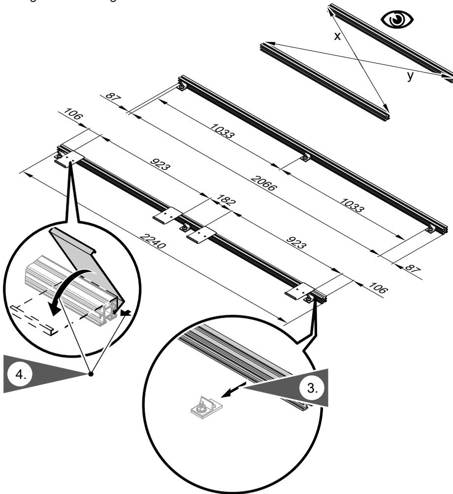
Fig. 22 Maximum deviation from dimensions  $x$  and  $y$  10 mm
