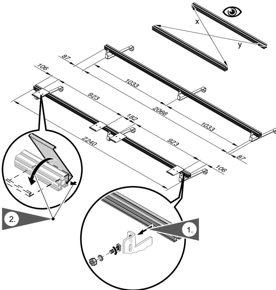
Fig. 18 Maximum deviation from dimensions x and y 10 mm
