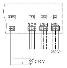
The 0 – 10 V hook-up provides an additional set boiler water temperature:
