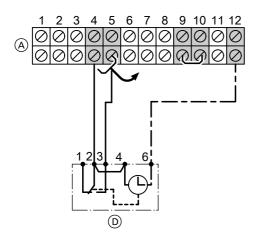
(A) Terminal strip inside the Vitotronic 100, type KC3 D Vitotrol 100, type UTA
