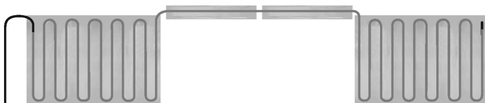
Fig. 5 Adaptation for recesses, obstacles, furniture, etc.
