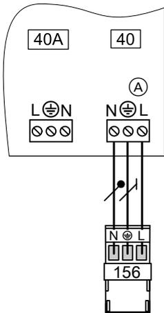
Fig. 15 Example: Power supply with plug 156
