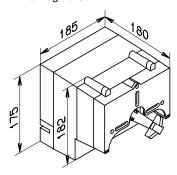
The mixer regulator is mounted directly on the Viessmann mixer DN 20 to 50 and R  $\frac{1}{2}$ " to  $\frac{1}{4}$ ".
