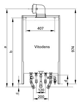
Existing water connections have identical dimensions.
