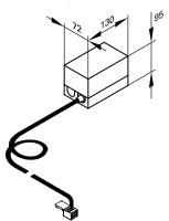
The temperature limiter is installed into the heating flow and switches the heating circuit pump OFF if flow temp. is too high. With connection cable (approx. 4 m long) and system plug.
