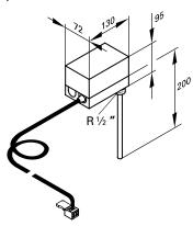
The temperature limiter is installed into the heating flow and switches the heating circuit pump OFF if flow temp. is too high. With connection cable (approx. 4 m long) and system plug.
