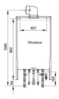
Existing water connections have identical dimensions.
