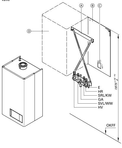
Illustration: Gas-fired combination boiler connection
