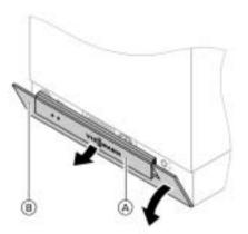
Lift up the cover (A), and pivot the control unit flap (B) down. All boiler controls are located behind the control unit flap.
