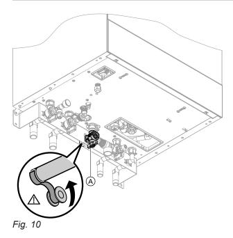
When carrying out any work on gas connection fittings, counterhold with a suitable tool. Never transfer any forces to the internal components.
