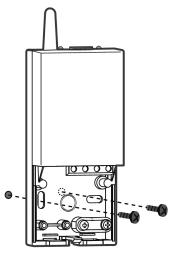
To feed the cable through the back panel, break out the pre-punched hole and guide the cable through it.
