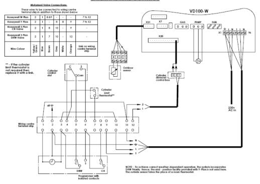
Option 2: outdoor sensor with internal time control (Viessmann accessories)
