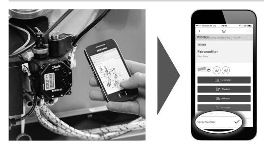
The wearing parts that have to be serviced can be identified and ordered via the Viessmann spare part app.
