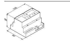
Mounting rail installation TS35 to DIN EN 50 022, 35 x 15 and 35 x 7.5.
