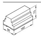
Mounting rail installation TS35 to DIN EN 50 022, 35 x 15 and  $35 \times 7.5$ .
