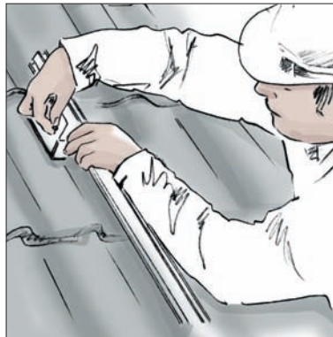
6. Attach rails to brackets. 7186230
