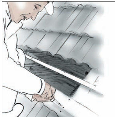
3. Fix timber battens to joists. 7188482/7188483/7186230
