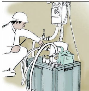
C. Pump fluid in using floor standing or hand-fill pump, and vent the system.
