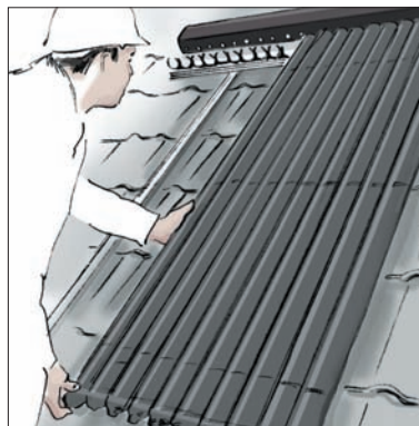
9. To insert tubes rotate & push gently until they lock into position. 7188857
